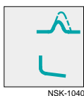
带电磁式过电流的隔离开关 Non-automatic circuit-breakers with magnetic overcurrent release
