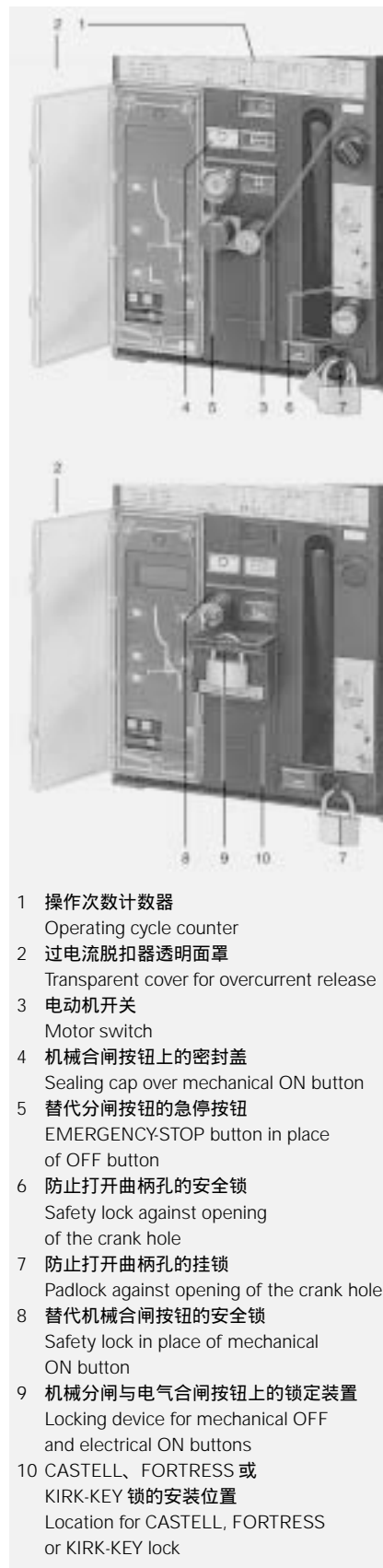
图 22 分闸、合闸和锁定装置 Fig. 2/22 Opening, closing and interlocking devices
