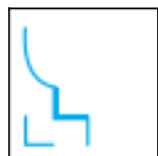
短路短延时保护(“z”) Short-time-delay short-circuit protection (“z”)
