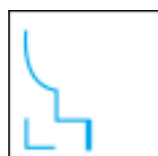
短路瞬时保护(“n”) Instantaneous short-circuit protection (“n”)
