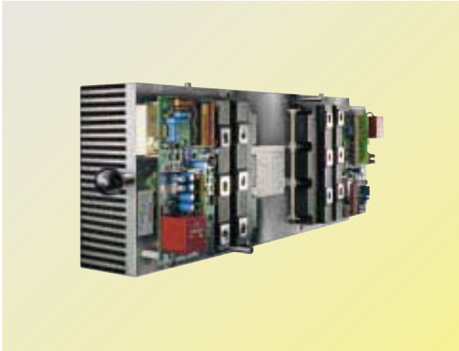
Fig. 2/3 Modular and service-friendly: Air-cooled HV-IGBT Power-Card of the motor-side drive converter
