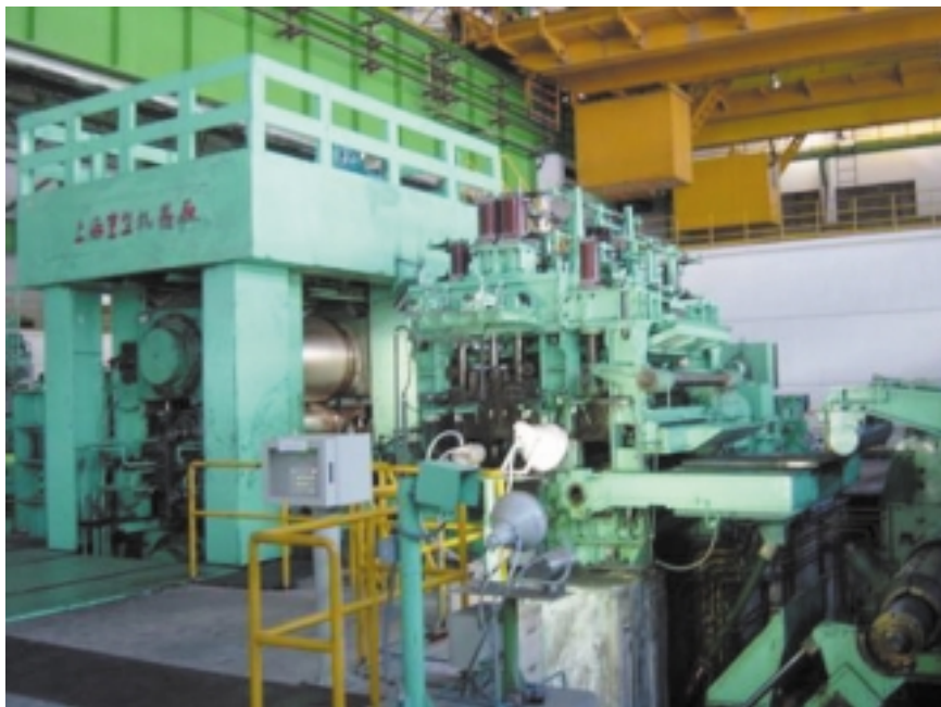
分卷平整机组的主要设备开卷机、矫直机、平整机 Main devices of decoling and temper rolling unit: decoiler, straightener, skin pass mill
